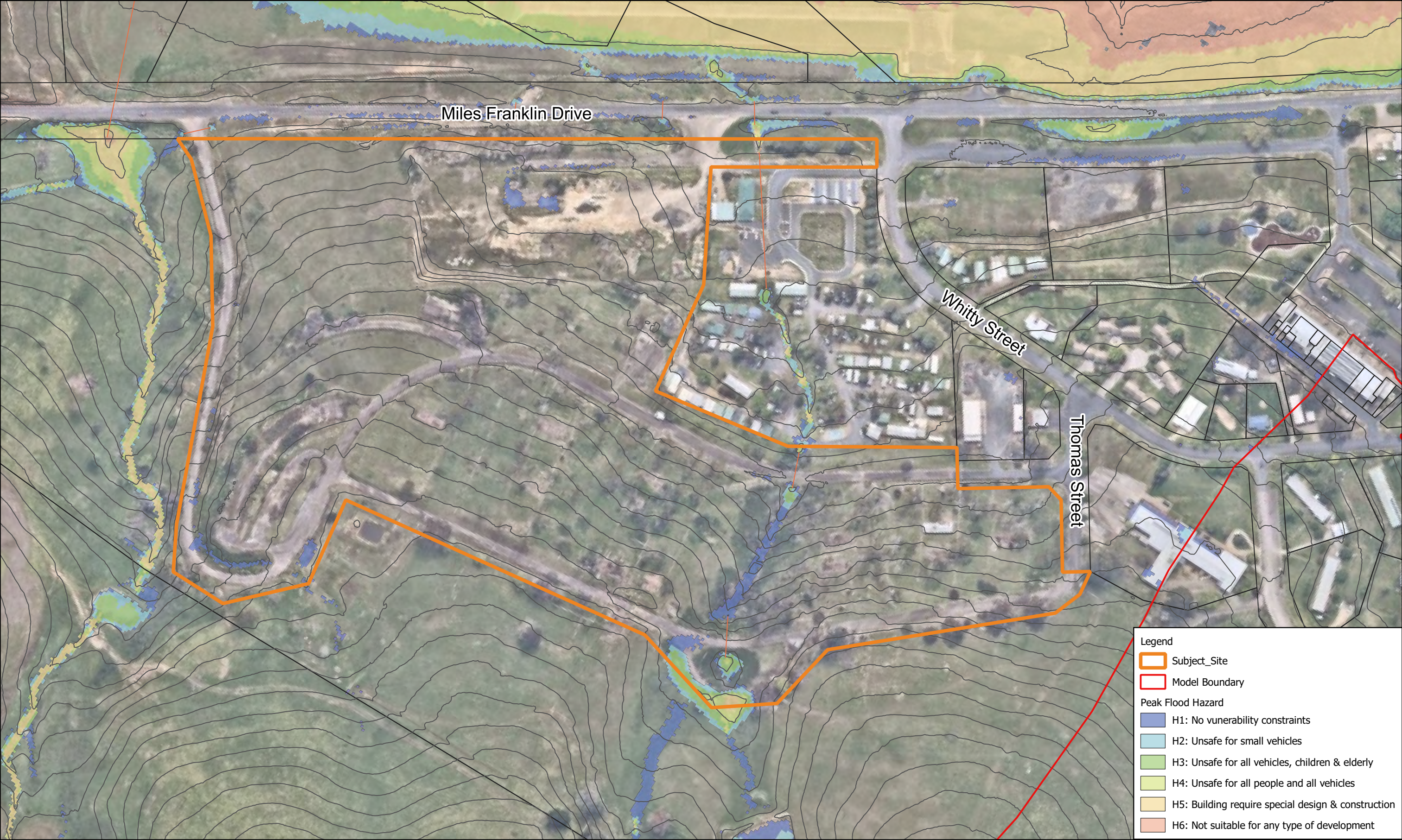
Title: Talbingo West Masterplan - Miles Franklin Drive, Talbingo Existing Scenario - Peak Flood Hazard 5% AEP Event
