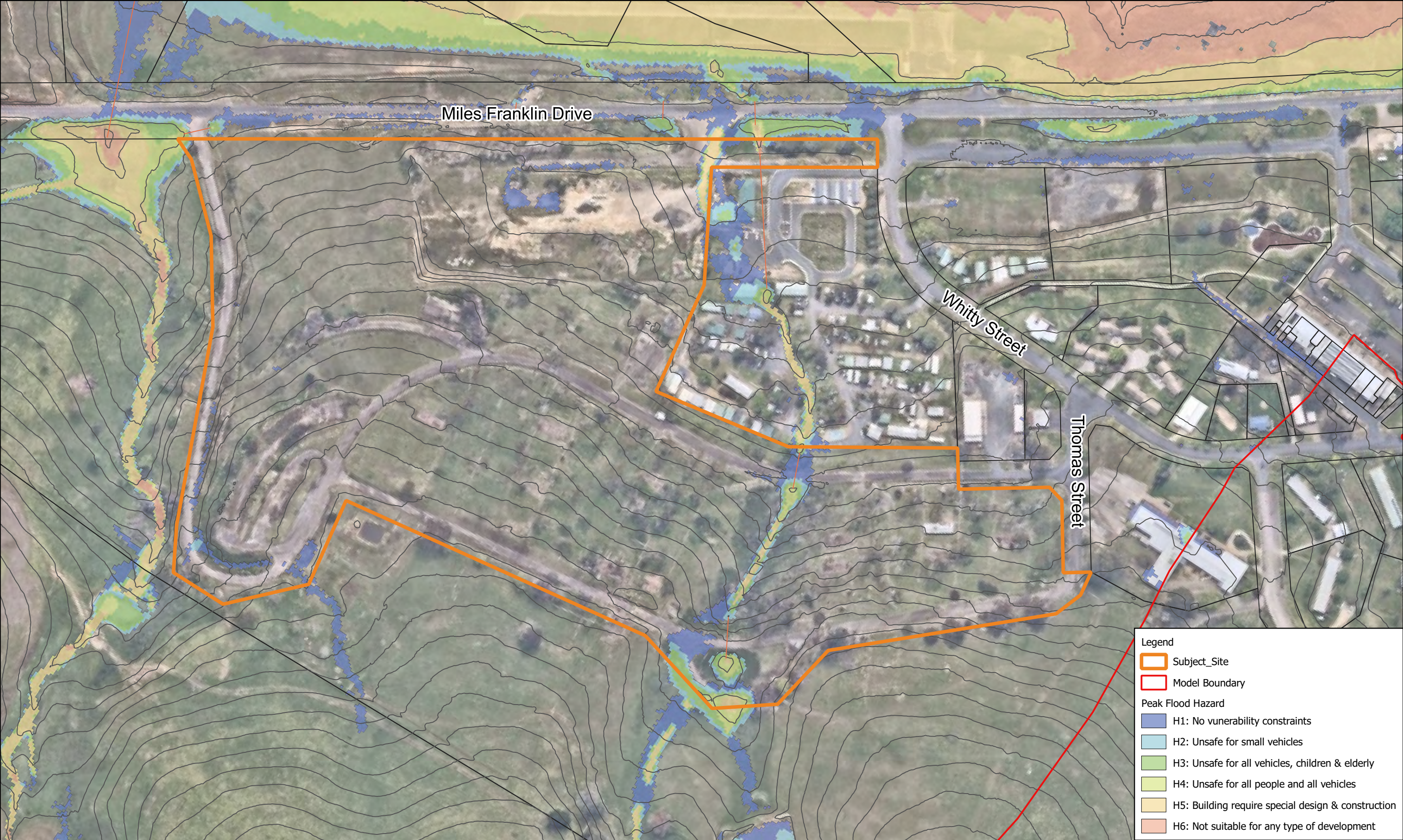
Title: Talbingo West Masterplan - Miles Franklin Drive, Talbingo Existing Scenario - Peak Flood Hazard 1% AEP Event
