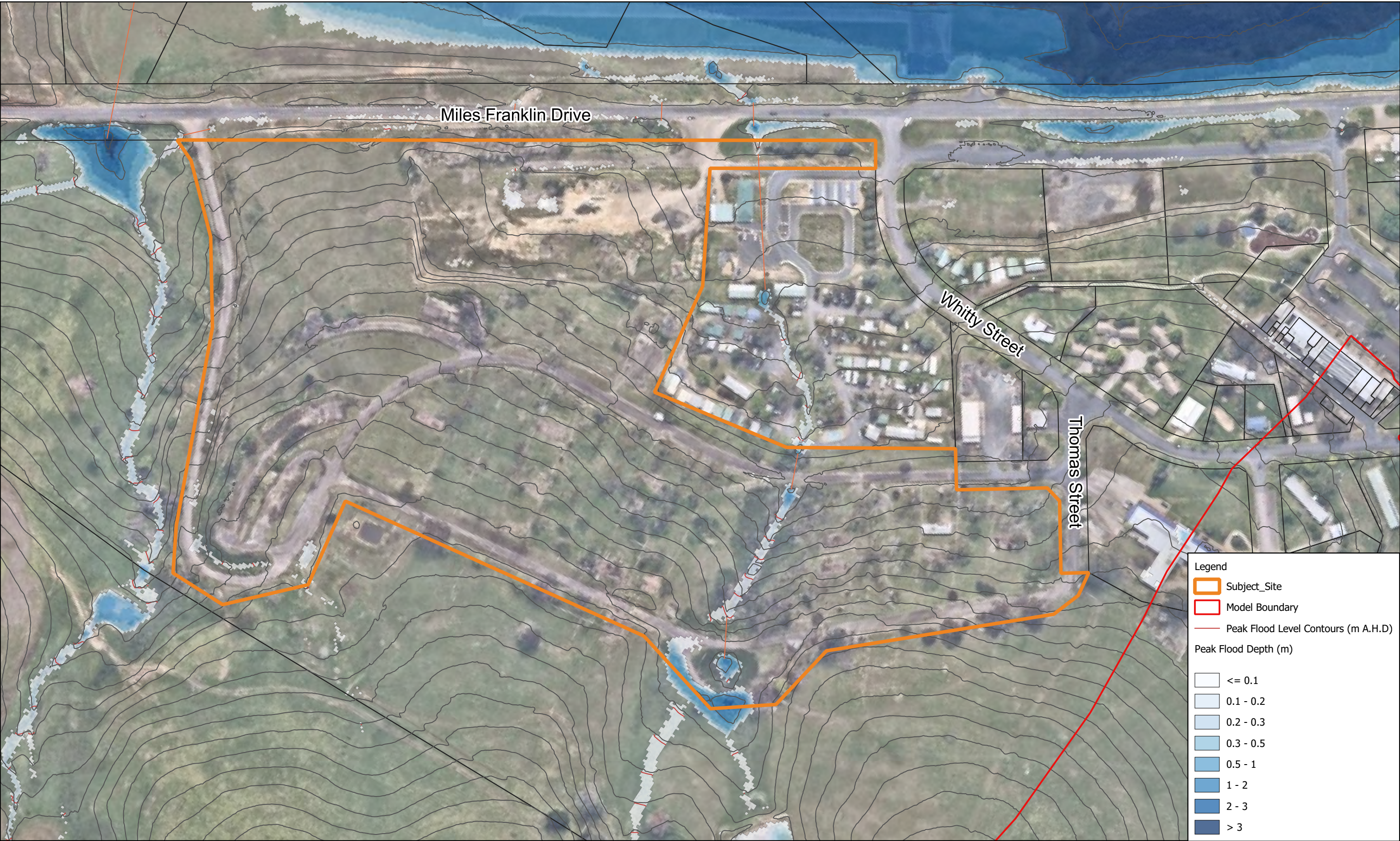
Title: Talbingo West Masterplan - Miles Franklin Drive, Talbingo Existing Scenario - Peak Flood Depth 5% AEP Event
