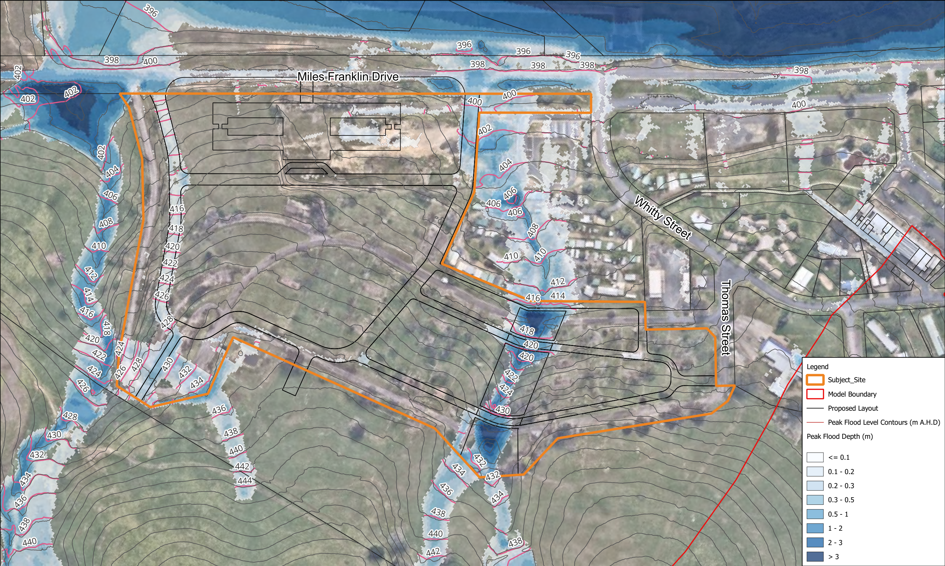
Title: Talbingo West Masterplan - Miles Franklin Drive, Talbingo Proposed Scenario - Peak Flood Depth PMF Event
