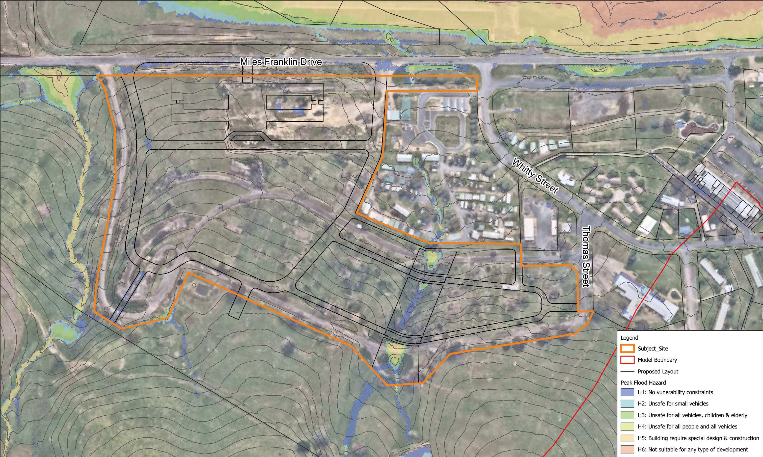
Title: Talbingo West Masterplan - Miles Franklin Drive, Talbingo Proposed Scenario - Peak Flood Hazard 5% AEP Event
