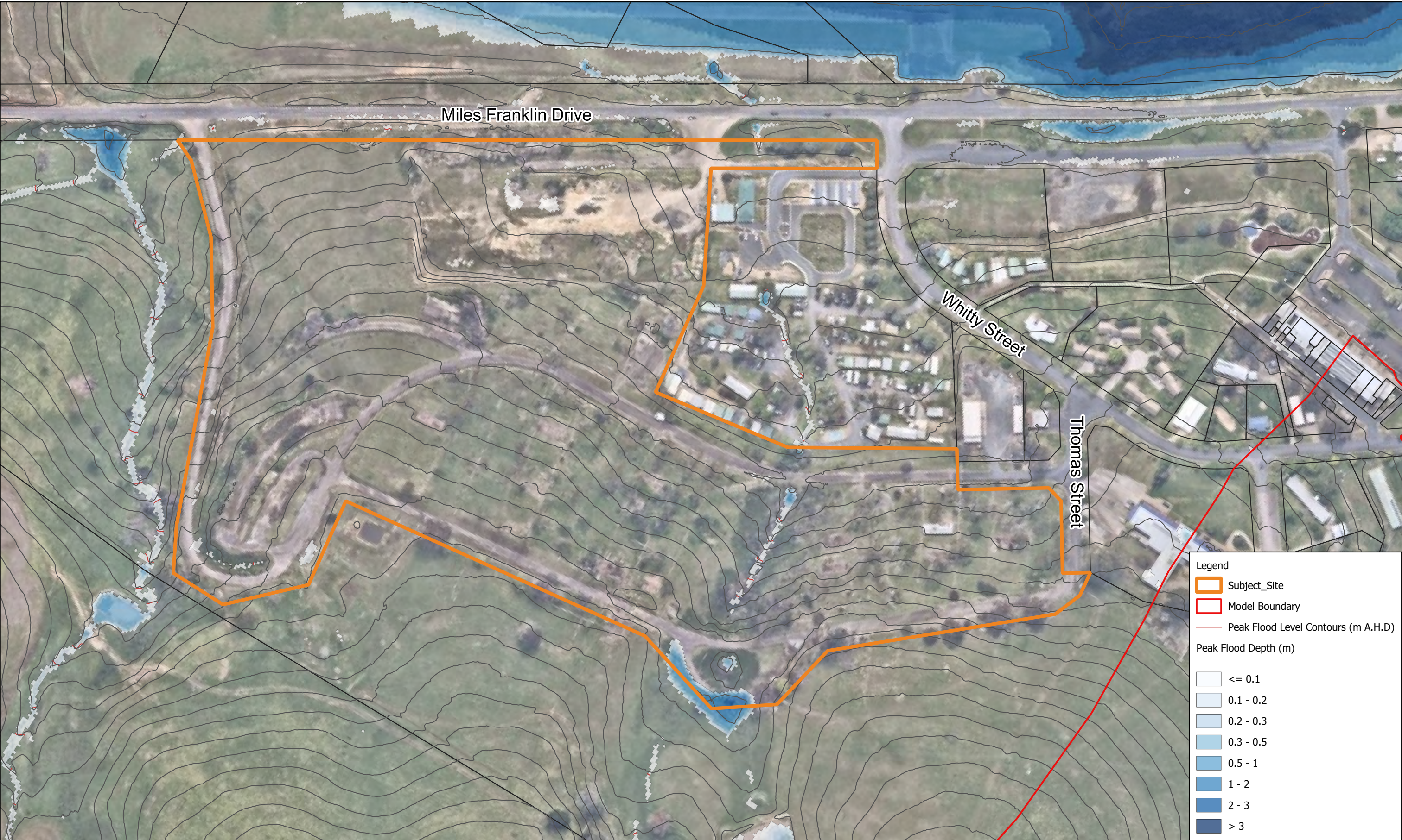
Title: Talbingo West Masterplan - Miles Franklin Drive, Talbingo Existing Scenario - Peak Flood Depth 20% AEP Event
